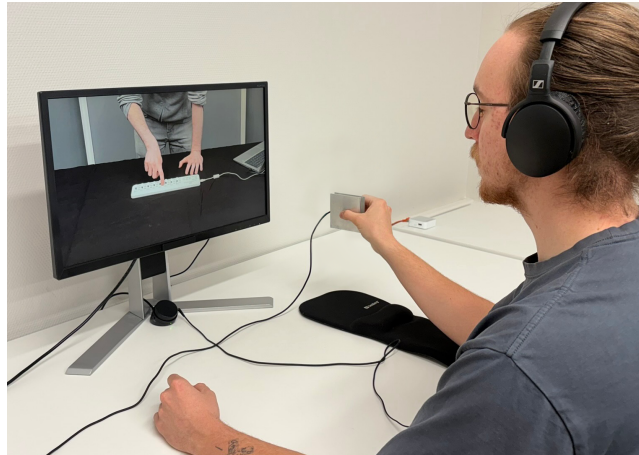
Figure 1: Experimental setup. The participant held the grip force sensor between thumb, index, and middle fingers, with the forearm resting on a cushioned support.
