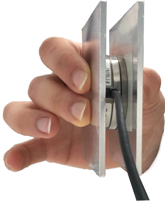
Figure 2: Grip force sensor. Close-up of the ATI Mini40 grip force sensor, mounted with two custom aluminum contact plates, held between thumb, index, and middle fingers.
