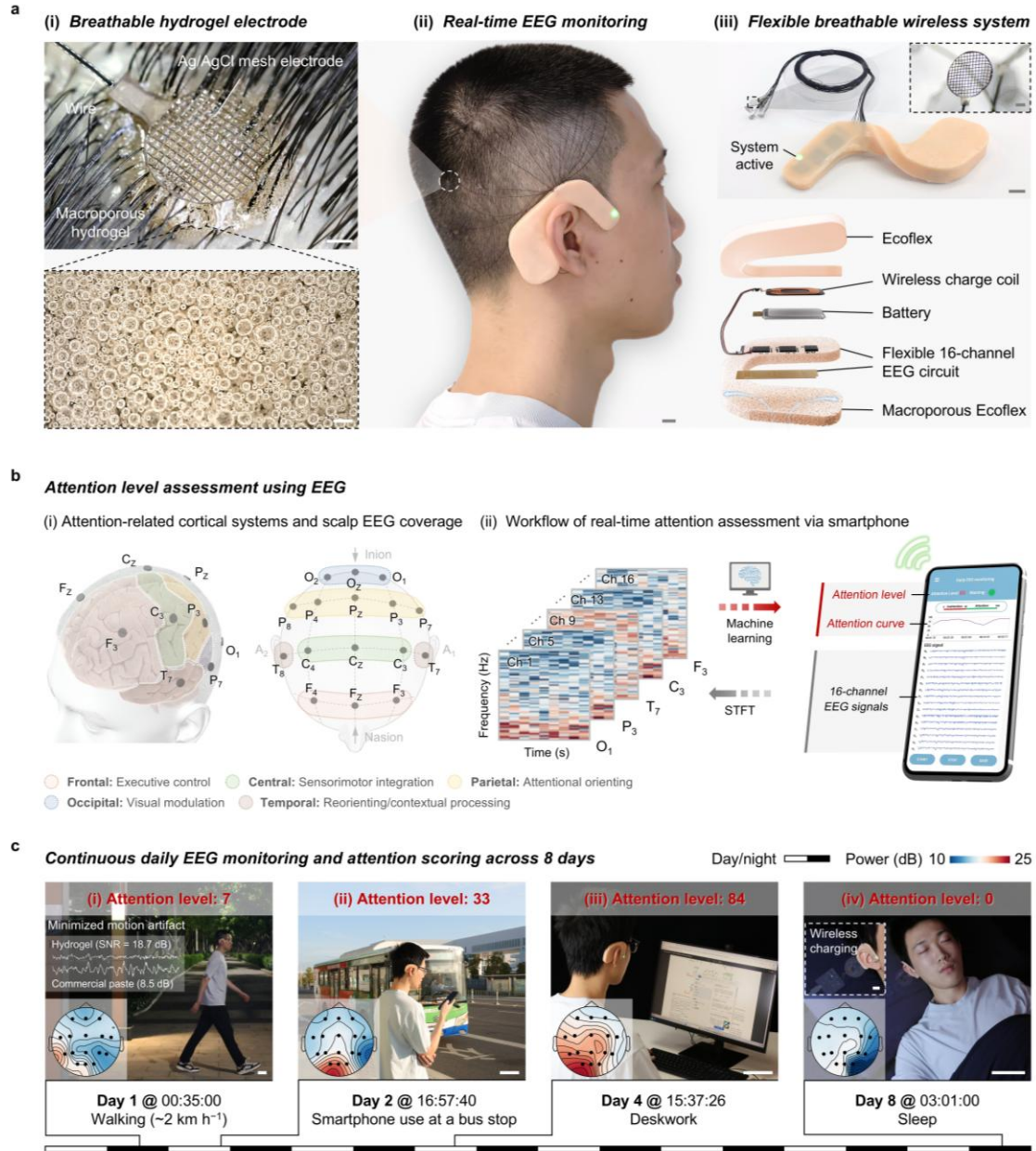
Fig. 1. Breathable wireless EEG system with macroporous hydrogel electrodes enabling 8-day continuous daily brain recording and attention assessment. a , (i) Photograph of an in situ-gelled macroporous hydrogel integrated with an Ag/AgCl mesh electrode in conformal contact with the hair-bearing scalp (top) and a magnified view of the hydrogel architecture (bottom). Scale bar, 2 mm (top); Scale bar, 500 \mu\text{m} (bottom). (ii) On-body demonstration of the earhook wireless EEG system. Scale bar, 1 cm. (iii) Photograph of the flexible and breathable 16-channel earhook wireless module connected to Ag/AgCl mesh electrodes via thin commercial wires (top) and exploded view of the earhook wireless module (bottom). Scale bar, 1 cm. Inset: magnified view of the Ag/AgCl mesh electrode. Scale bar, 10 \mu\text{m} . b , Attention-related cortical systems and scalp EEG coverage used in this study. (i) Schematic of cortical systems involved in attentional control, including frontal control-related processes, central-midline engagement and monitoring, parietal attentional orienting, occipital visual-attention modulation, and lateral temporal
