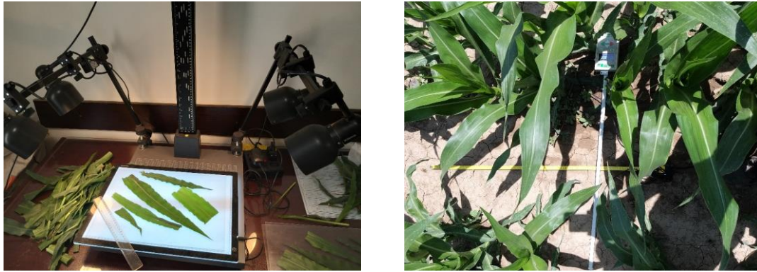
Figure 4. Leaf area was measured using the Delta-T leaf area meter
