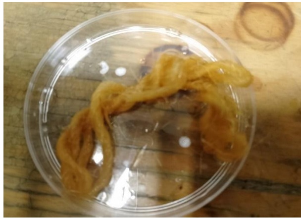
Fig. 2: Sample Preparation – Soaking of Sisal fibre in distilled water and sodium hydroxide
