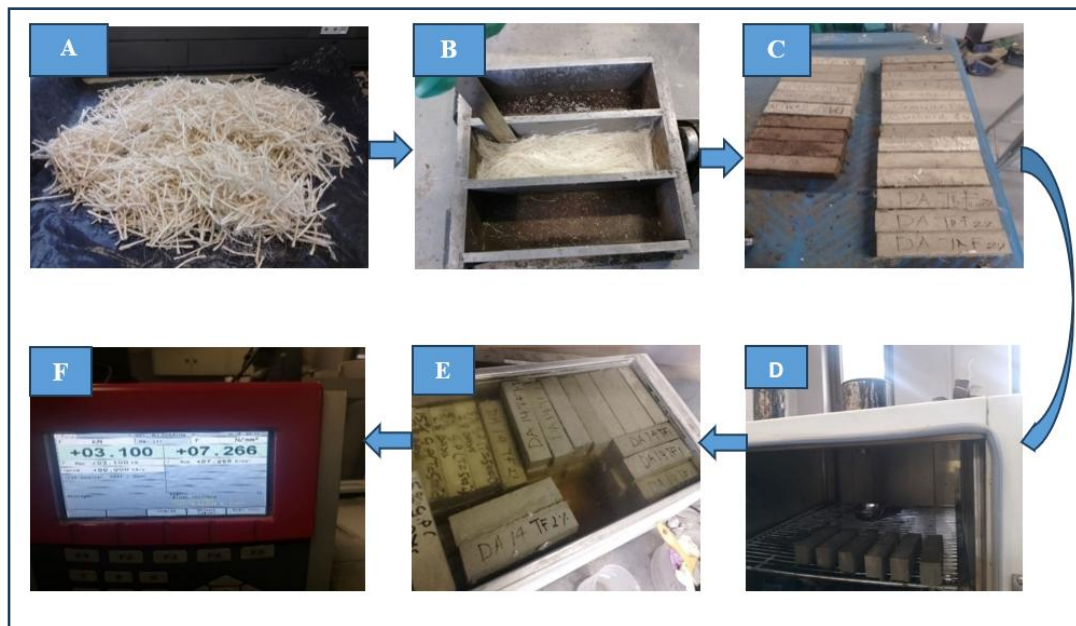
Fig. 5: (A)Processed sisal fiber, (B) Casting of mortar, (C) Curing of mortar, (D) Mortar samples in oven (E) Samples left out to cool and dry (F) Result of mortar testing at seven
