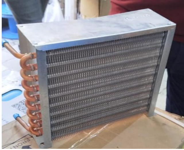
Figure 9: Finned-tube evaporator used for thermal regulation of the electrolyzer system
