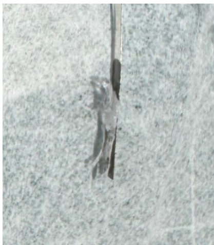
Figure S3 Photo of delaminated PFSA (same functional group as Nafion) ionomer-based coating on Ag|AgBr RE.
