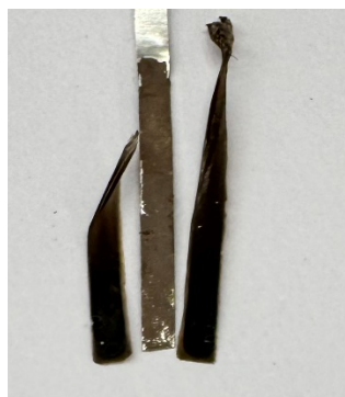
Figure S4 Photo of a delaminated and carbonated coating layer on Ag|AgBr RE composed of a of fluorinated ethylene propylene (FEP) polymer and perfluorosulfonic acid (PFSA) ionomer after annealing up to 265 °C, based on the previous reported method 2 .
