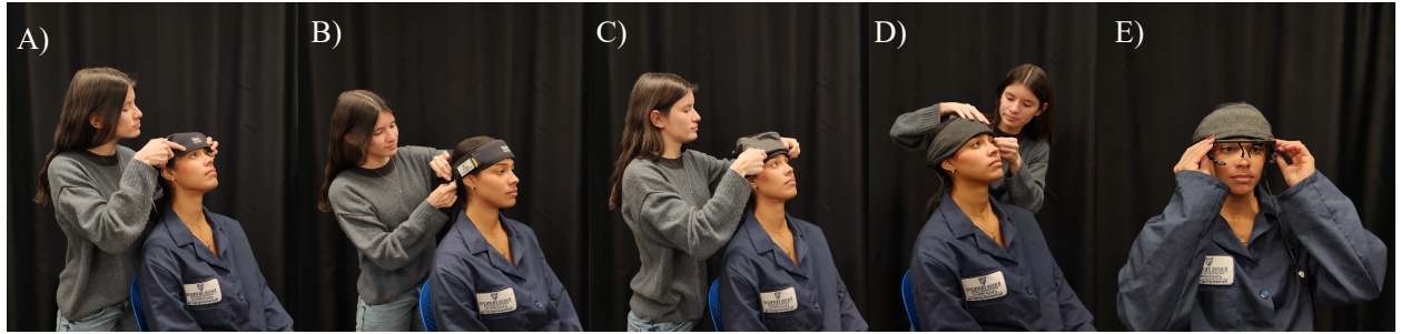
Figure S1: Sequential procedure for fitting the fNIRS headband and eye-tracking glasses prior to data collection. (A) Initial placement of the fNIRS headband over the participant's forehead. (B) Alignment of the headband relative to anatomical landmarks. (C) Securing and tensioning the headband to ensure stable contact. (D) Placement of an elastic cap to further stabilize optodes during data collection. (E) Placement and adjustment of the eye-tracking glasses.
