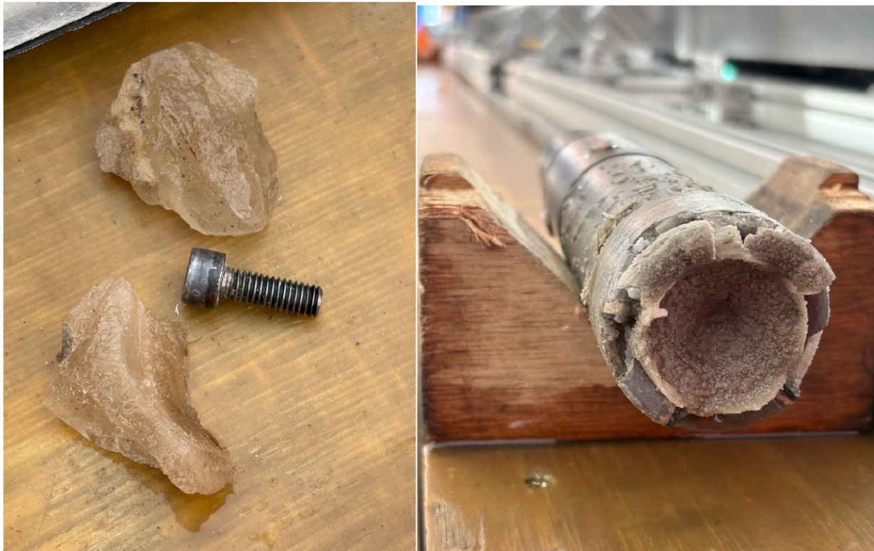
829 830 Figure S3_4: Bag n. RD3-25-26. Left: The two pieces that fell out at the top of the drill. Right: refrozen material in and around the 831 drillhead.
