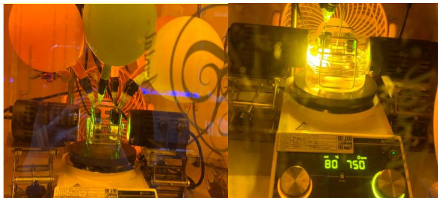
Figure S2. Typical reaction setup for irradiation experiments: 23 °C (left), 80 °C (right).
