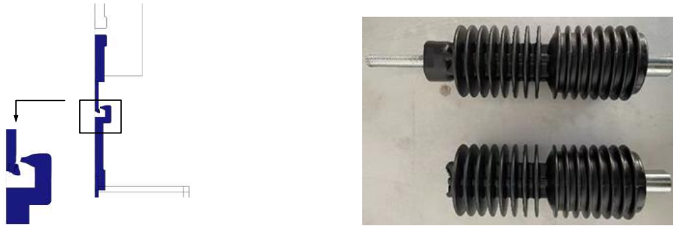
(a) The damage in the stress concentration area of the insulating rod accumulates until it breaks. (b) On-site picture of tie rod fracture
