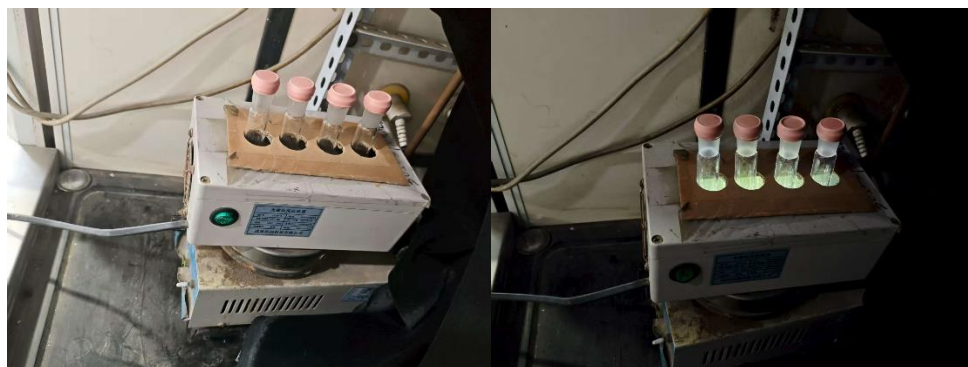
Figure S1. General setup for the reaction. A variable temperature photoreactor equipped with 12 W blue LEDs ( \lambda_{\text{max}} = 365 \text{ nm} ) was used for the reaction.
