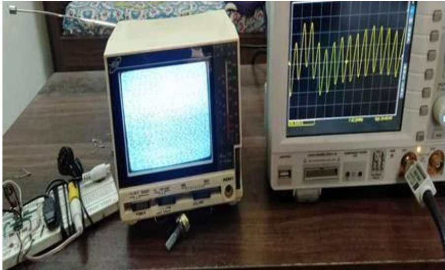
Fig. 20 Solution 1: stable 67.25 MHz RF carrier on oscilloscope (right); analog television shows static due to PAL/NTSC incompatibility (left)
