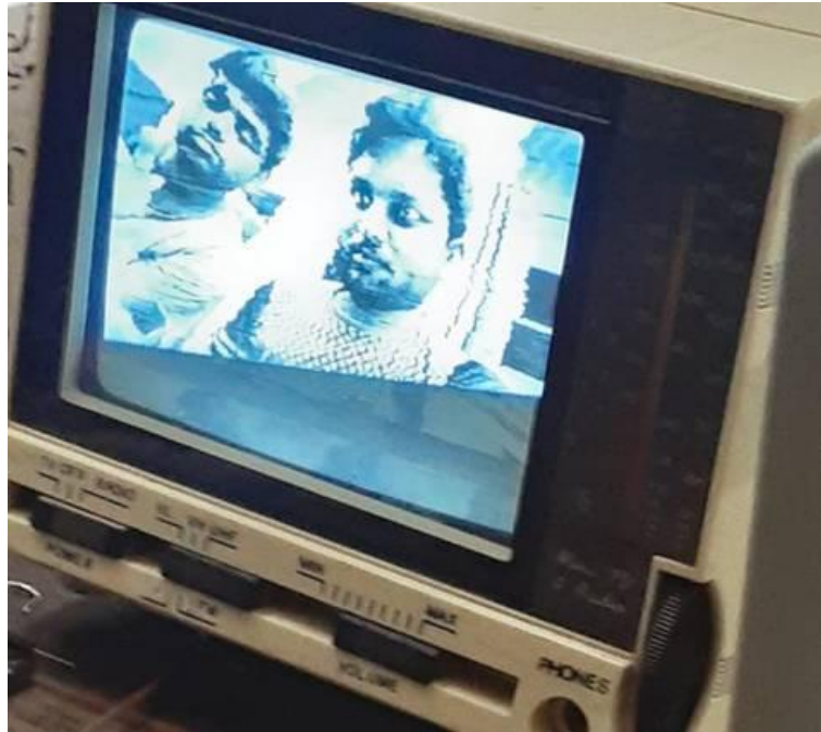
Fig. 21 Solution 2: clear real-time video on analog PAL television — two observers visible, confirming successful end-to-end wireless video transmission
