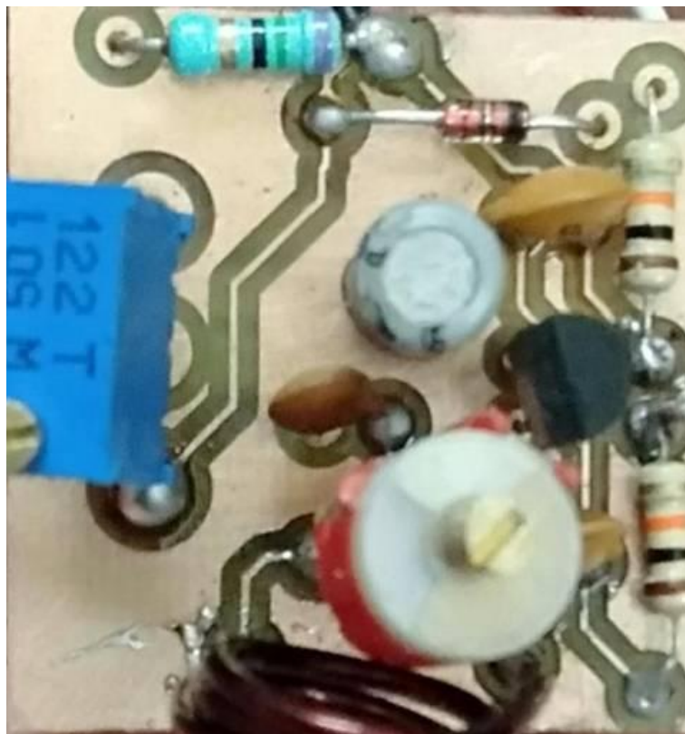
Fig. 18 Solution 2 PCB fully populated with all discrete components including variable capacitor (blue, top-left) and custom-wound inductor (bottom-left)
