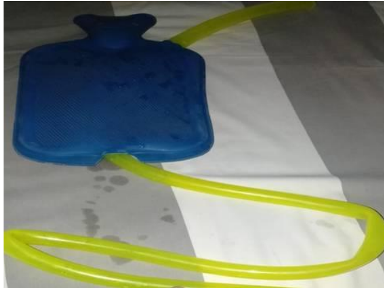
Fig. 2 Artificial body model: rubber hot-water bottle connected to flexible plastic tubing, used to simulate the GI tract during prototype testing
