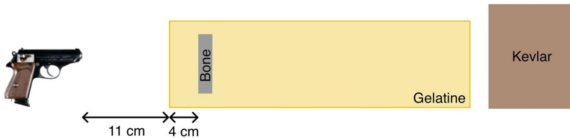
Figure 6: ballistic test setup used for both ammunition types. A carton box filled with Kevlar was placed behind the gelatine/bone model in case the bullet perforates it completely.
