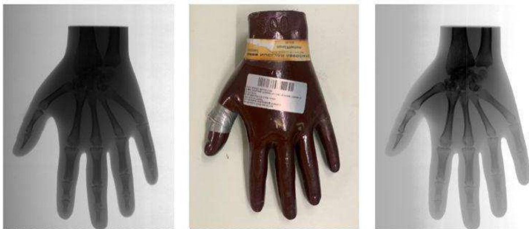
Fig. 12. Anatomical hand phantom is used to simulate a more realistic contrast examination situation. Victoreen Nuclear Associate Hand Phantom 76-634 x-ray image taken by SyncBox controlled TDI detector x-ray scanner. 0.5 mm aluminum filtration has been used.
