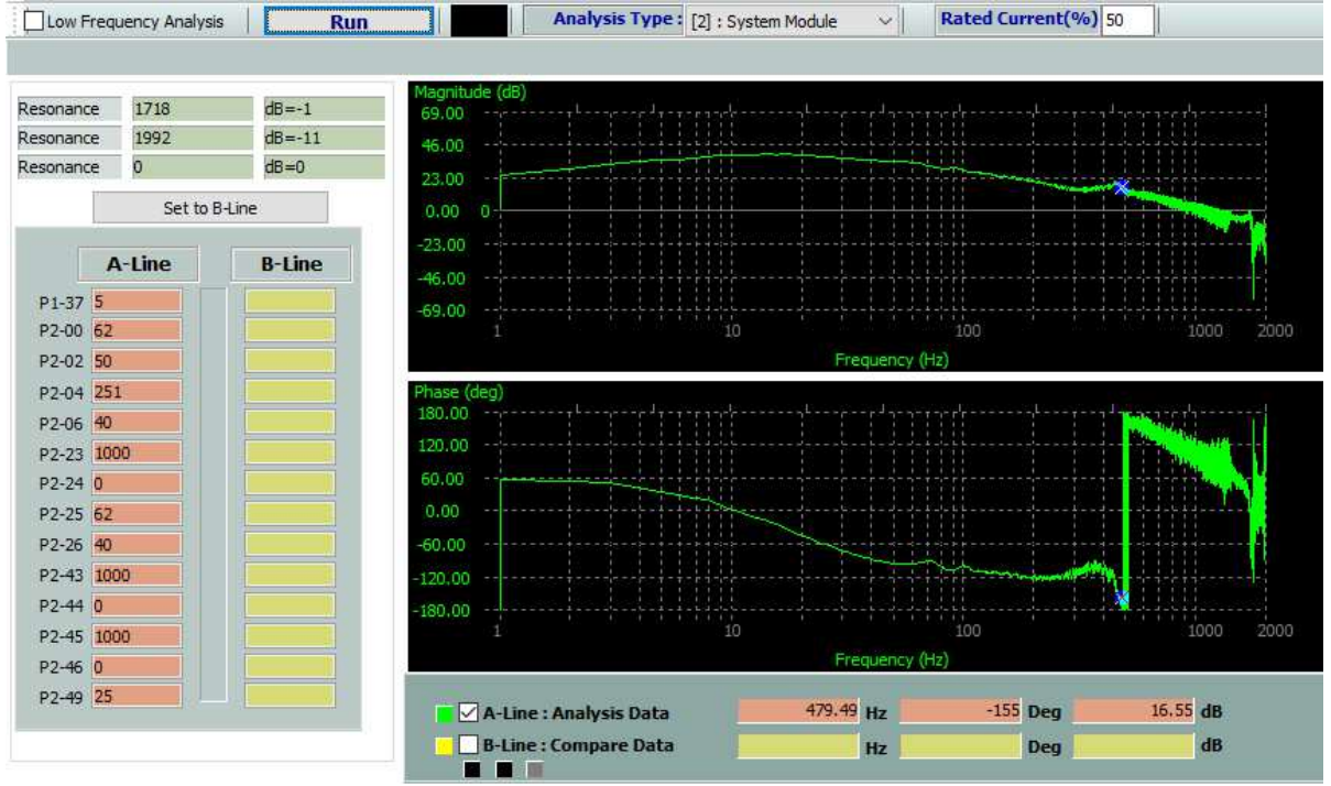
Figure 10 Bode diagram of the control loop. The gain bandwidth is around 500 Hz and the zero phase happens around 10 Hz.
