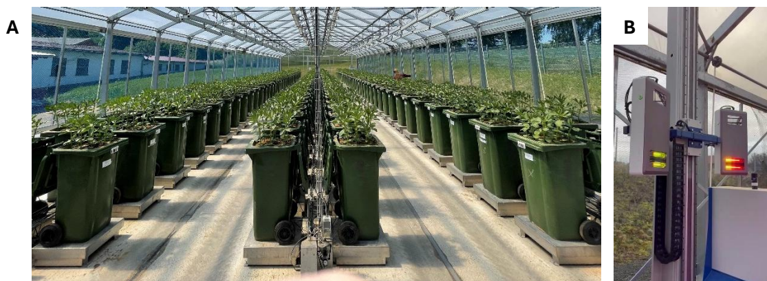
Fig. 1 High-throughput phenotyping platform “Droughtspotter XXL” comprising 240 containers, each with a rootable volume of 120 liters, housed under a foil greenhouse providing semi-controlled environmental conditions ( A ). Automated phenotyping with a multispectral 3D scanner enabled high-resolution, non-destructive monitoring of plant growth and canopy development throughout the experiment ( B ).
