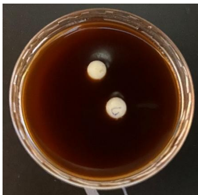
Fig. 3: The specimens were immersed in staining solution at room temperature for 28-days test period.
