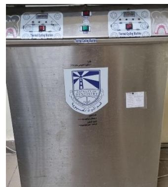
Fig. 2: The specimens were then subjected to aging by thermal cycling in which A total of 10,000 cycles in the water bath was applied to simulate one year of oral use.
