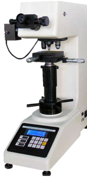
Fig. 8: The Vickers hardness numbers for the tested samples were calculated using a Vickers micro-hardness tester under 500 Newton of force.
