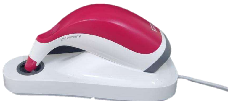
Fig. 4: A digital spectrophotometer has been used to determine the precise and reliable shade matching for the specimens.
