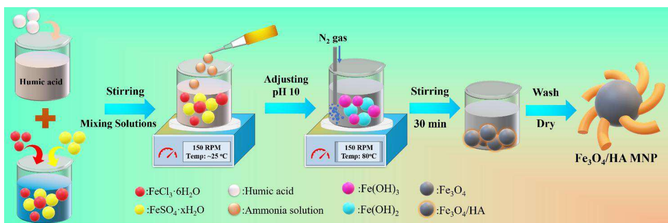
Figure 1. Schematic preparation of \text{Fe}_3\text{O}_4/\text{HA} MNP via co-precipitation method
