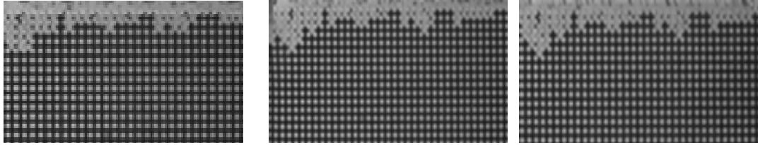
(d) Second cycle, fluid flow at 10 min injection, 5 min shut-in, and 10 min shut-in (low permeability)
