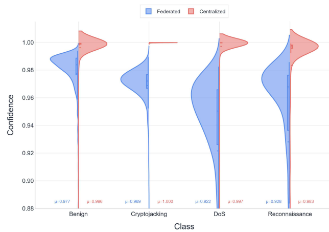
Figure 10. Split-violin plots comparing prediction confidence distributions between federated (left half, blue) and centralized (right half, red) models per attack class. Both models achieve near-unity confidence, with the centralized model showing marginally tighter distributions.
