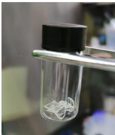
Fig. S58. Pieces of the plastic cup (105.6 mg) in a vial prior to hydrogenolysis
