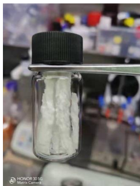
Fig. S66. Pieces of expanded polystyrene foam (109.3 mg) in a vial prior to hydrogenolysis
