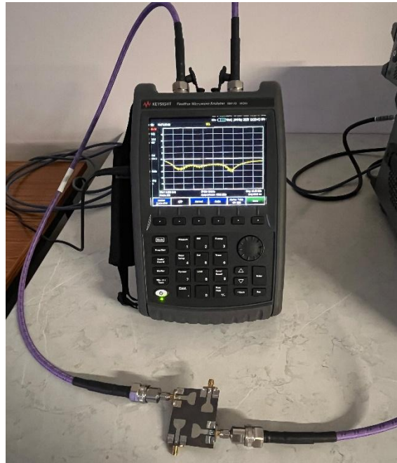
Figure 7. The proposed MIMO antenna validated using VNA
