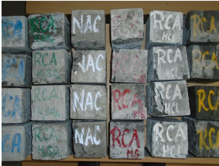
Figure 9 Failure Patterns of Cubes under Compressive
