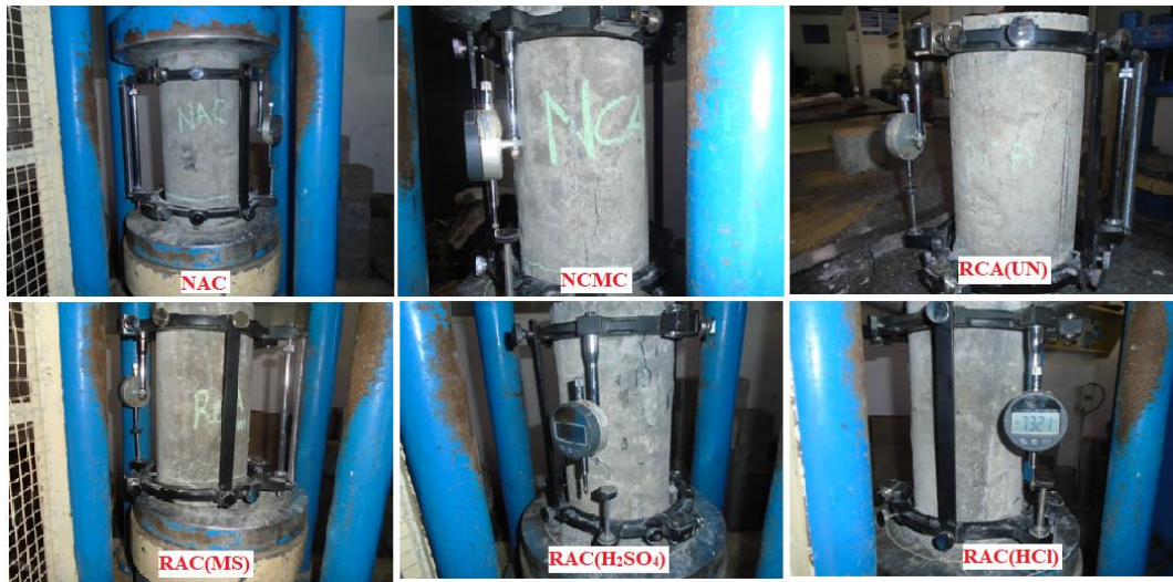
Figure 15 Failure Pattern of Modulus of Elasticity
