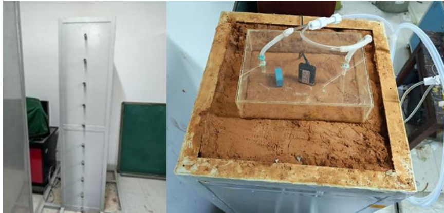
Fig. 1 Physical diagram of the rectangular prism soil column simulation apparatus and radon accumulation chamber connection
