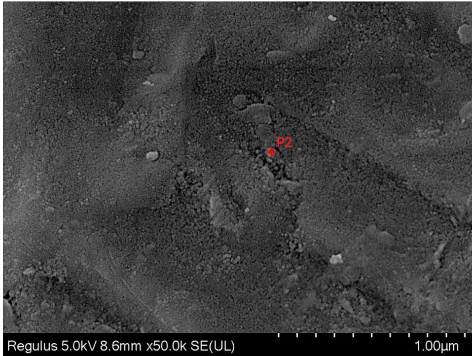
Figure S3. SEM image of the localized corroded region on glaze surface shows the nanoscale particles with varying packing densities.
