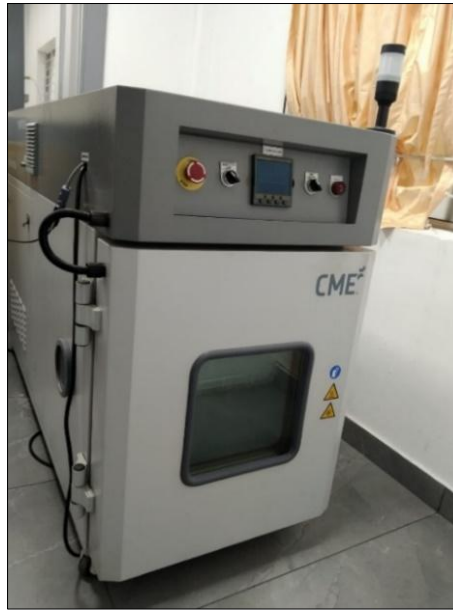
Figure 5. Environment chamber used for ageing studies
