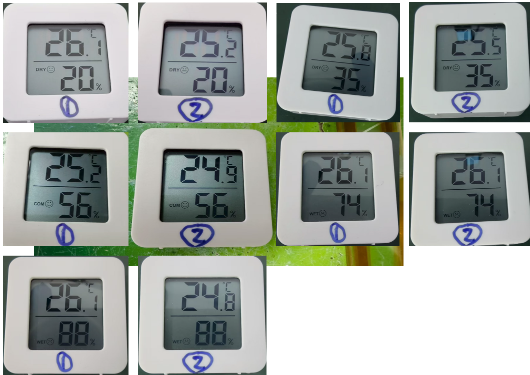
Supplementary Figure 40 | Two commercially available humidity sensors were used to measure the actual humidity of the air entering the test chamber.
