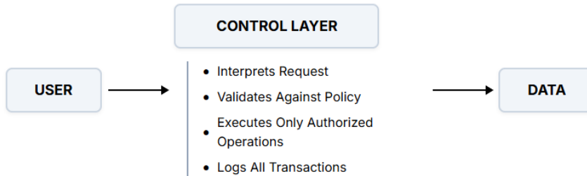
Fig. 1 Traditional versus Positive Data Control (PDC) data access. In traditional architectures, users interact directly with data systems and policy checks are often applied post hoc. In the PDC model, a control layer mediates all requests, interprets user request, validates policy compliance, and logs decisions before any operation reaches the data layer.
