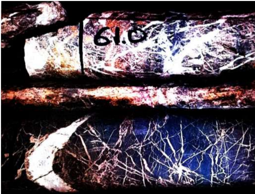
Figure 13: Drill core (DV1701; ~61.0 m downhole) showing dense baryte-siderite stockwork within dark siltstone.
