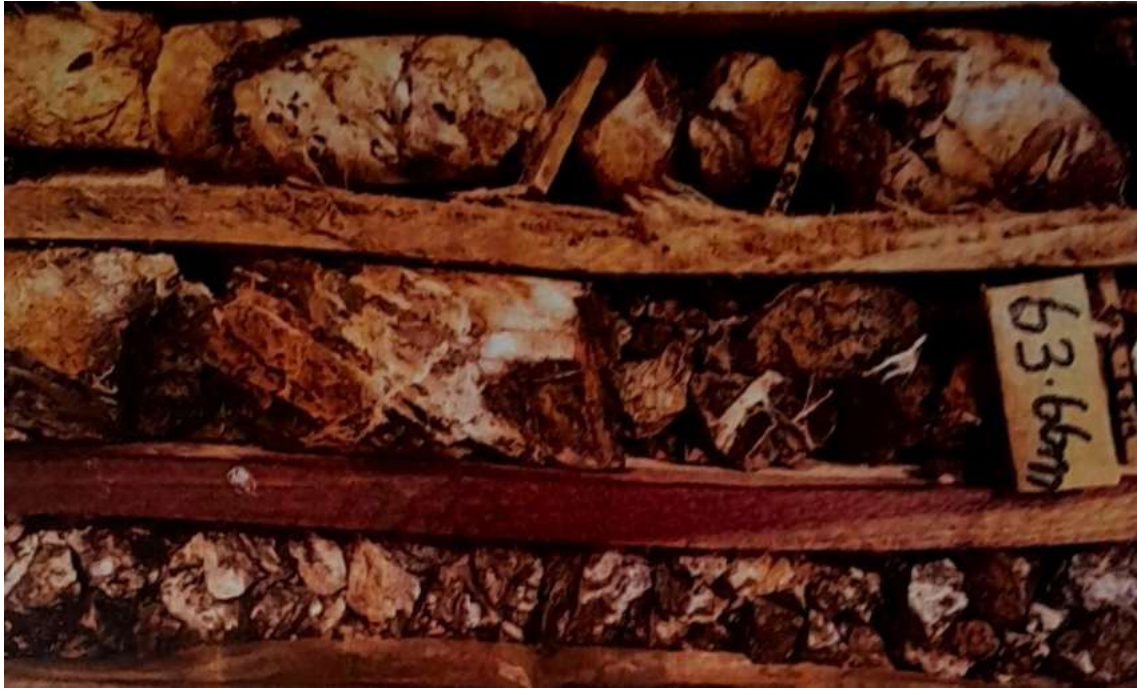
Figure 24: DV603 Baryte veins in gossan with fine quartz stockwork
