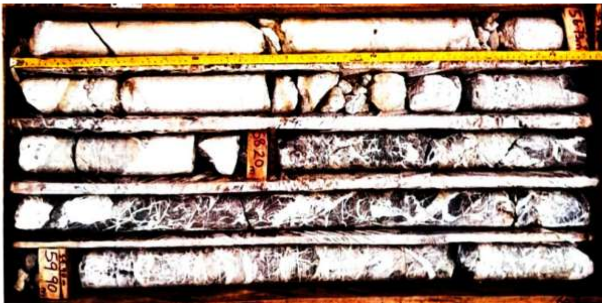
Figure 12: Core photograph of the DV1701 main lode intersection showing massive and brecciated baryte within the shear zone.
