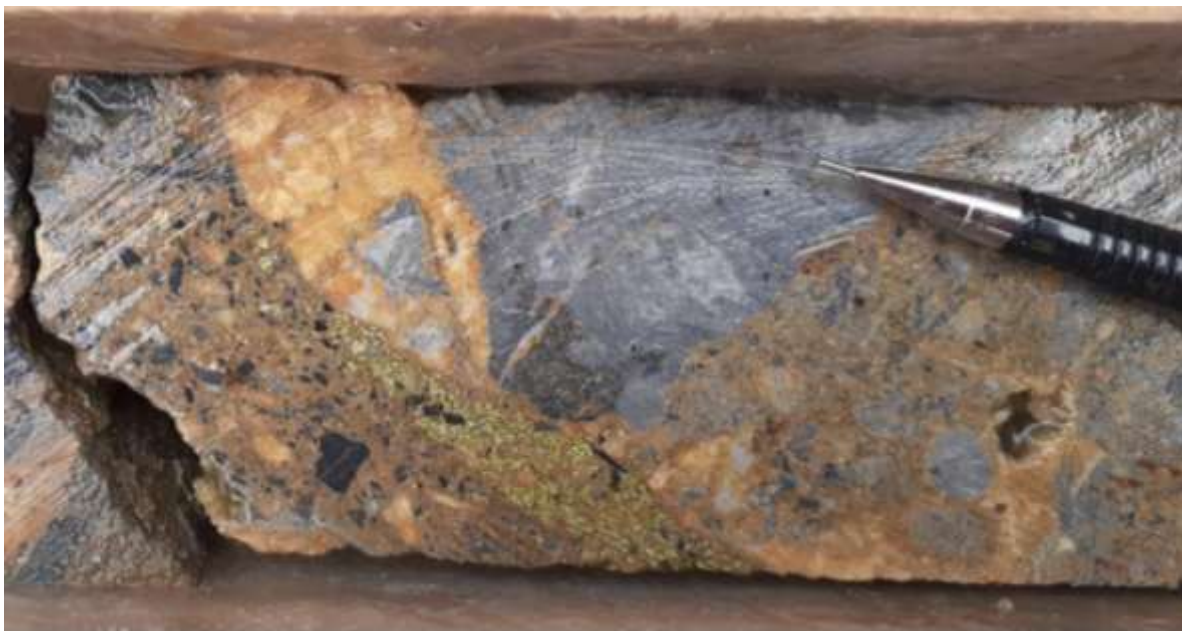
Figure 14: Chalcopyrite in younger siderite breccia, DV1702, 68.3m
