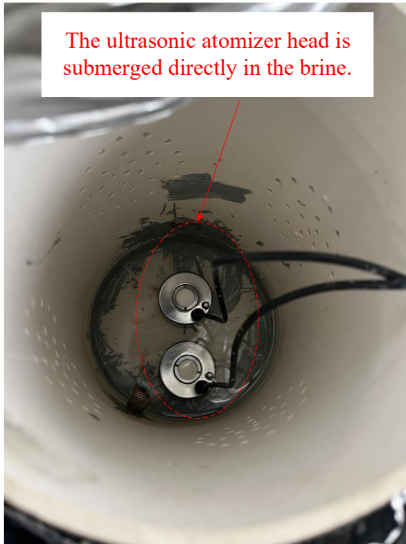
Supplementary Materials Fig.1 Comparison photograph of the brine atomization unit (a) and the milk atomization unit (b)
