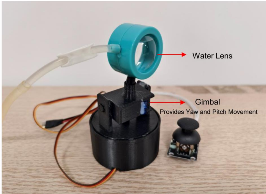
Supplementary Fig. 21: Water lens and rotation device for simulating joint changes in corneal curvature and gaze direction.
