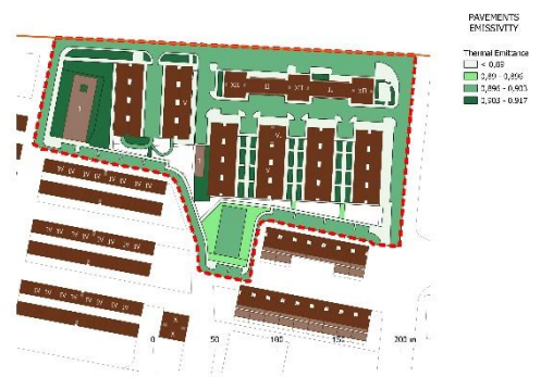
Figure 17. Mapping of the thermo - optical properties of urban surface materials. Aerial view and measures of emissivity of pavements in Orcasur district
