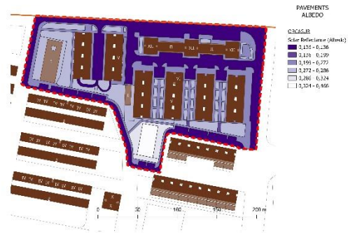
Figure 16. Mapping of the thermo - optical properties of urban surface materials. Measures of solar reflectance of pavements in Orcasur district
