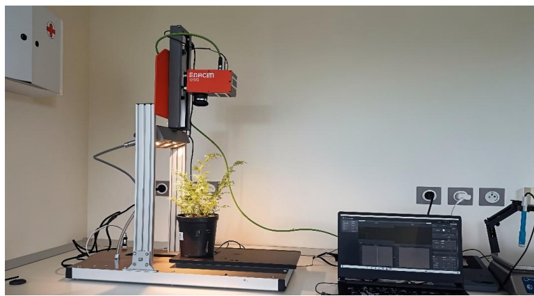
Fig. 2. The experiment site at ICARDA in Rabat, Morocco, using hyperspectral camera measuring a line of 1024 pixels with 448 spectral bands on chickpea plant pot.
