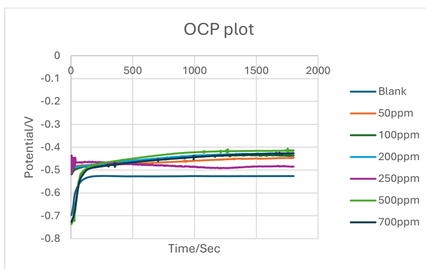
Figure 4. Time-dependent open circuit potential E_{ocp} of mild steel in 0.5 M \text{H}_2\text{SO}_4 in the presence of Aglaonema leaf extract, orange peel extract, and grape seed extract.
