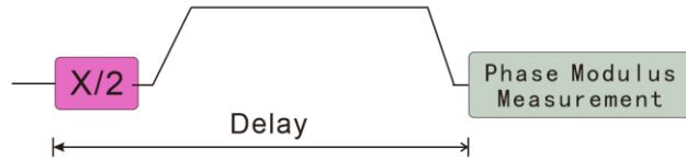
Figure S8. The measurement circuit for extracting dephasing time at various detuning points. We first apply an X/2 gate to initialize the qubit in a superposition of |0\rangle and |1\rangle , and then bias the qubit to different frequencies for a certain time. Then we bias the qubit back to measure its phase modulus.
