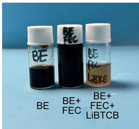
Figure S13 Digital photo of different electrolytes after storage at 50 °C for 15 days.
