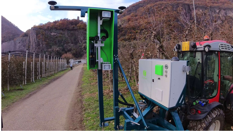
166 Fig. 1 PhenoMobile mounted on tractor at Auer, Italy, in December 2024. The platform integrates 167 two RGB cameras, two GNSS antennas, two flash units, and one LiDAR sensor.
