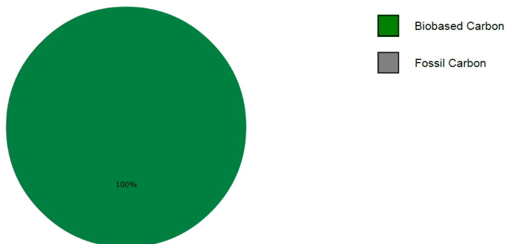
Fig. 2 Radiocarbon verification by ASTM D6866 [17] of renewable content in the microbial monomer
