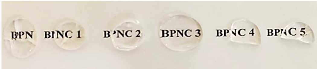
Figure 6: Borate-based bioactive glass samples with compositions (65-x) \text{ B}_2\text{O}_3 + 15\text{P}_2\text{O}_5 + 20\text{Na}_2\text{O} + x\text{CaO} (mol%), where x = 0 to 15. Samples are labeled BPN and BPNC1–BPNC5 based on CaO content.
