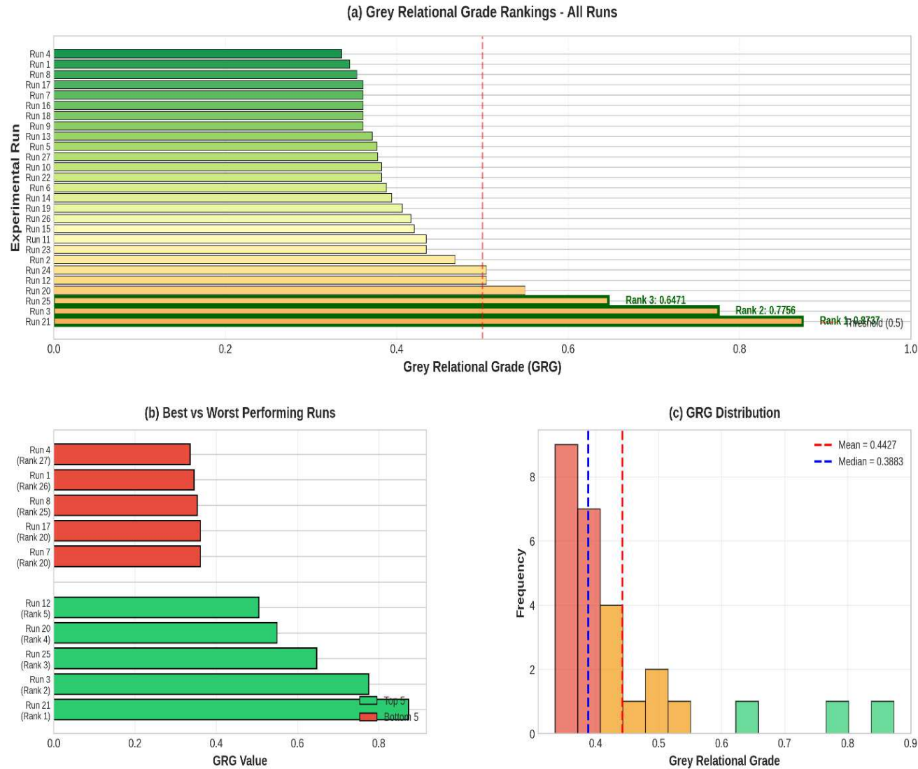
Figure 12: Comprehensive Grey Relational Analysis of Taguchi L27 optimization study. (A) Rankings: (a) GRG values for all runs with top three highlighted, (b) best vs. worst comparison, (c) GRG distribution.
