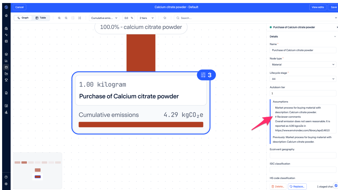
Figure S17: Example of a reviewer comment documented on a production graph node. The reviewer notes that overall emissions do not appear reasonable and cites a specific EPD as the documented reference value.
