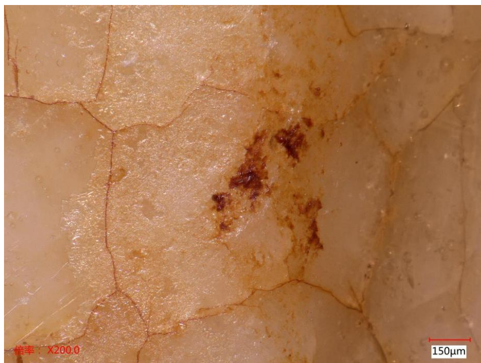
Supplementary Fig. 1. OM image of the protrusion on the outer wall of the transparent cream-glazed sample.
