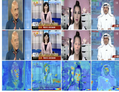
Fig. 4: Visualization of the localization process (top to bottom): Original frame, Manipulated frame, and Localization heatmap highlighting the forged regions.
