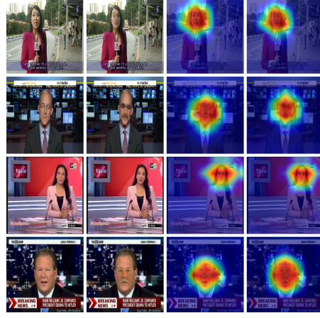
Fig. 3: Grad-CAM visualizations for EfficientNetB0 classification (left to right): Original image, Deepfake image, Grad-CAM overlay on original, and Grad-CAM overlay on deepfake.
