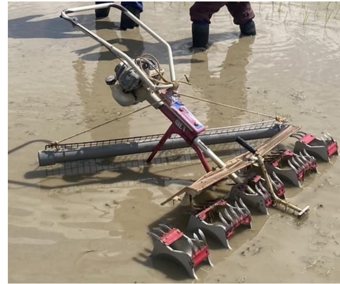
FigS2. The comparison of mechanical rotary weeder (M) and Chained-mechanical rotary weeder (MC) (Photograph)
