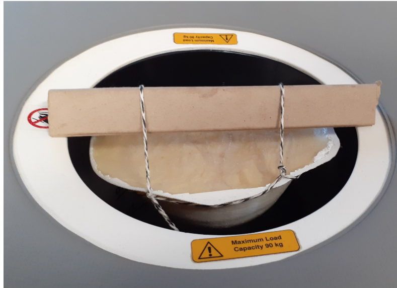
Fig. A4 Filled breast phantom suspended over BCT scanner.
