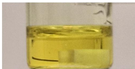
Figure S16. Precipitation points of water when added to the DMSO ink.
