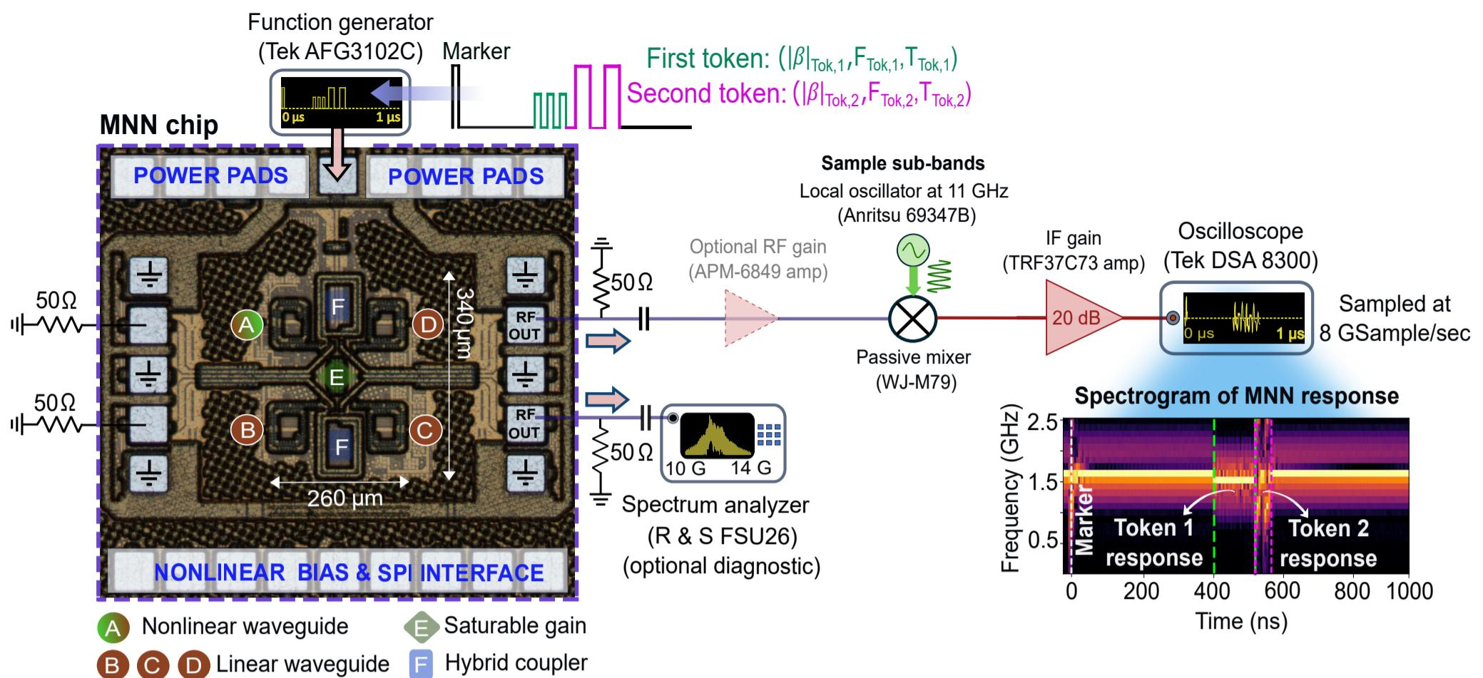
**b.** Experimental setup to record MNN's responses to fast data to assess p-bit behavior.
