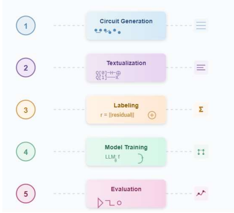
Fig. 1 Overall workflow of Quantum2Prompt. The pipeline consists of five stages: (1) Circuit Generation , where benchmark matrices and ansätze are used to generate VQLS circuits; (2) Textualization , which converts each circuit into a structured natural-language description; (3) Labeling , where the residual norm r = \|A|\psi\rangle - |b\rangle\| is computed via simulation or noisy sampling; (4) Model Training , where an LLM-based regressor f_\theta learns the mapping from text to residual; and (5) Evaluation , assessing generalization on unseen matrices and ansatz families. This design decouples quantum evaluation from surrogate learning, enabling low-cost prediction and initialization for VQLS.
