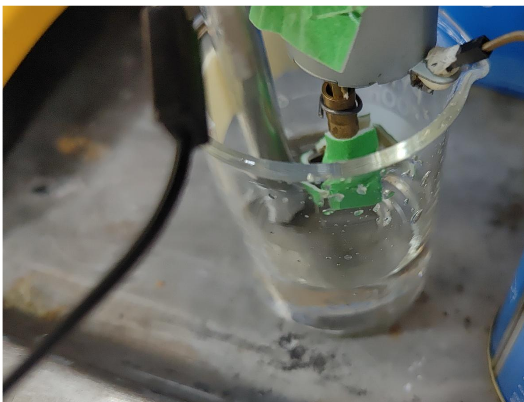
Figure S6: Pure Zinc rod was used in Pulse electrodeposition (Left), Servo motor was used to rotate the stainless steel substrate (Right)
