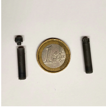
Fig. 2 Sample holder for VSM measurements. Left: A sample holder is 3D-printed from non-magnetic resin and consists of a 2 mm long hollow capillary (O.D. 5 mm, I.D. 3 mm) and a sealing cap. The capillary is filled with TEMPO. To measure the correct volume of TEMPO, the weight of the capillary and cap is recorded before and after filling with TEMPO. We use 1\text{g}/\text{cm}^3 as the density of TEMPO. Right: Example of a closed VSM capillary. The cap is further secured with epoxy glue.
