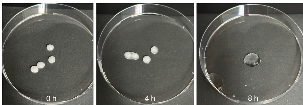
Supplementary Fig. 4 | Deliquescence of KOH pellet at ambient air under 40–50% RH at 25 °C after 4-h and 8-h exposure.
