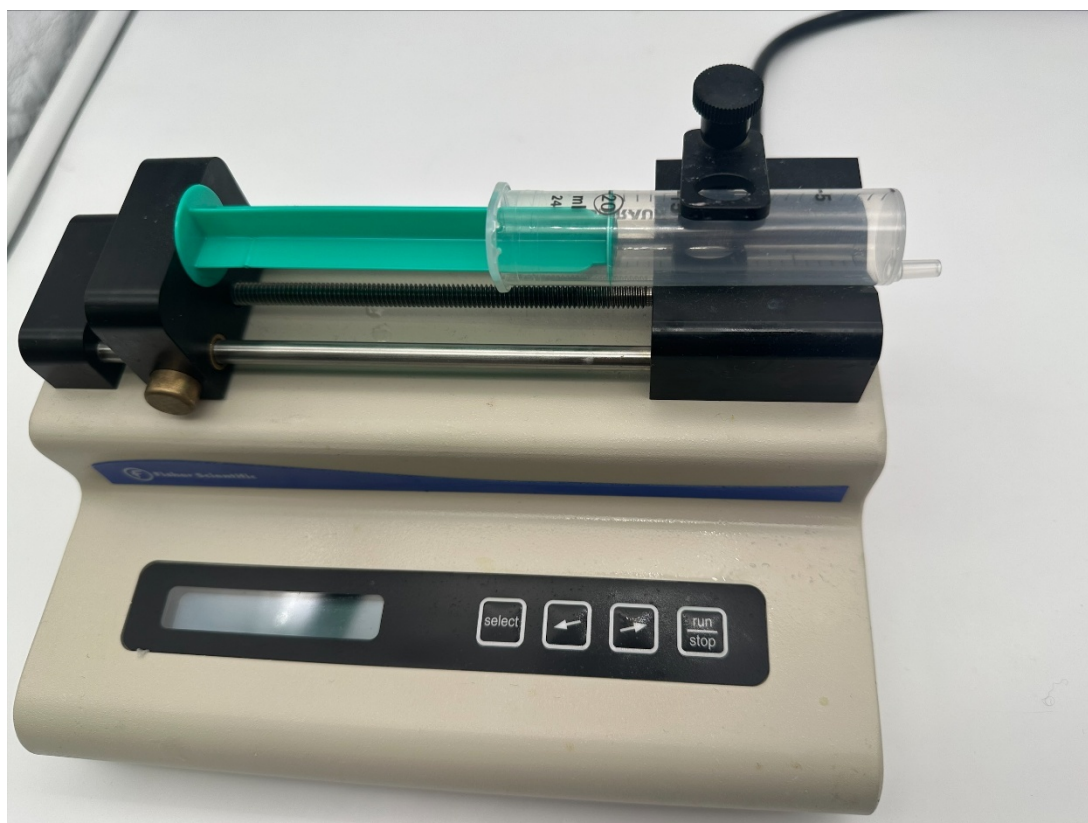
Supplementary Fig. 11 | The syringe pump for the generation of dry ice smoke with controlled flow direction and rate. 1 g of solid dry ice was mixed with 4 ml of distilled water inside the syringe. The flow rate was 420 ml h -1 .
