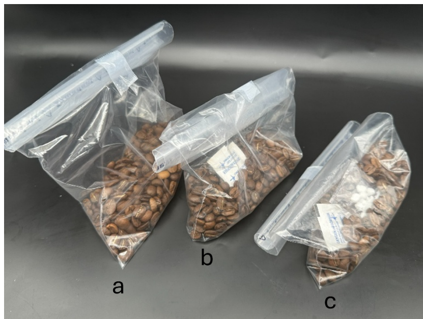
Supplementary Fig. 51 | Comparison of in-pack gas volume during coffee bean storage. Each bag contained 50 g of freshly roasted coffee beans. Commercial coffee packaging typically employs a one-way degassing valve to vent \text{CO}_2 while restricting \text{O}_2 ingress. To isolate the effects of gas capture, the freshly roasted beans were sealed without prior degassing or \text{N}_2 purging. In this valveless configuration, a commercial oxygen adsorbent was included to minimize the influence of residual \text{O}_2 on pouch swelling, for example, from lipid oxidation. a , Without any sorbent, the bag exhibited pronounced swelling, primarily due to \text{CO}_2 evolution and residual \text{O}_2 . b , With only the oxygen adsorbent, swelling was reduced but remained evident because \text{CO}_2 was neither vented nor captured. c , When both the oxygen adsorbent and \text{CO}_2 -capturing microbeads were included, the bag showed the smallest headspace volume, consistent with simultaneous \text{O}_2 removal and \text{CO}_2 sequestration by the microbeads 29 .
